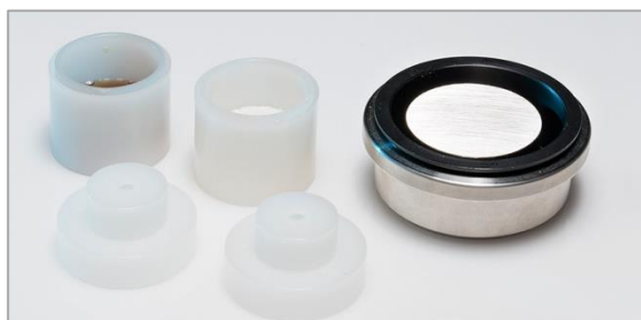
Figura 16 - Porta amostras do equipamento Epsilon 1 - Panalytical (MALVERN PANALYTICAL, 2019).
