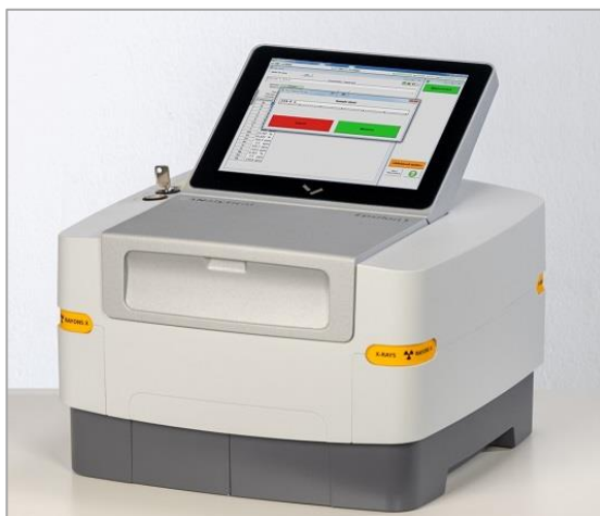
Figura 15 - EDXRF - Epsilon 1 – Panalytical (MALVERN PANALYTICAL, 2019).
