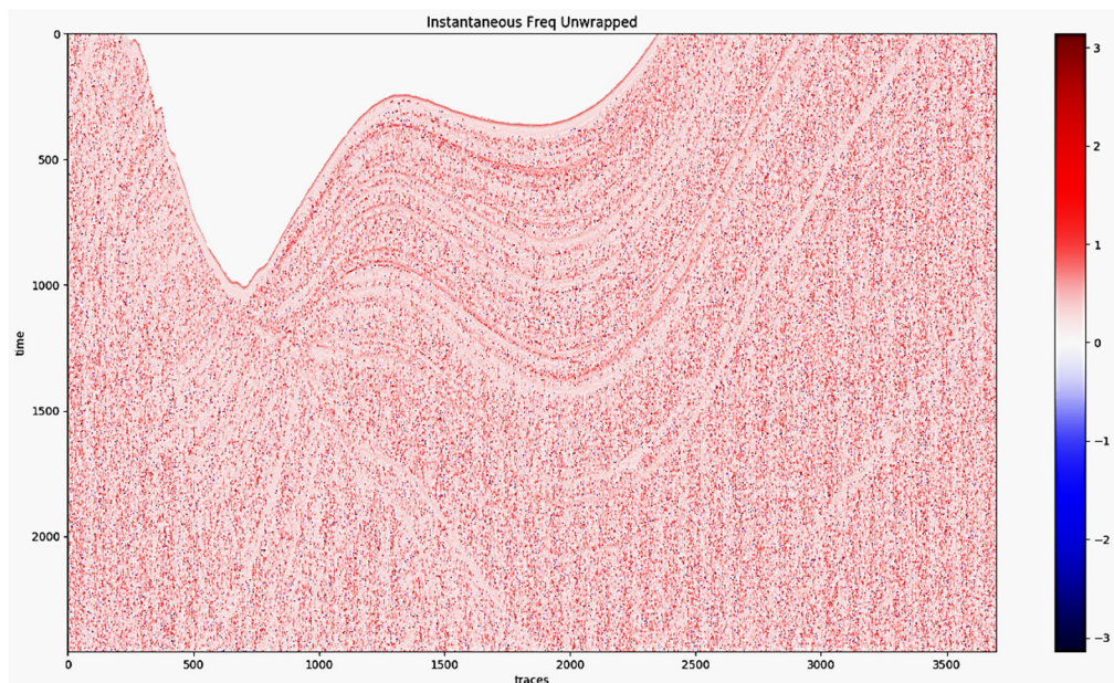
Figure 33 - The instantaneous frequency attribute computed from an unwrapped phase.
